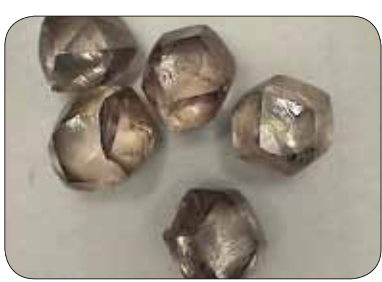
B: DODECAHEDRON Point angle 120 degree / Applications : SDD, Natural diamond-MDD
