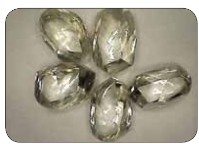
C: ELONGATED Oblong shape Applications : FDD cone type
